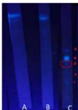
Figure 1. The results of the elution of the three mobile phase mixtures on UV lamp 366, mobile phase (A) : chloroform:ethyl acetate:methanol (8:8:4); (B) : chloroform:ethyl acetate:methanol: NH 4 OH (8:8:4:0.005); (C) chloroform:ethyl acetate:NH 4 OH (8:8:0.005). Stationary phase silica gel GF 254
