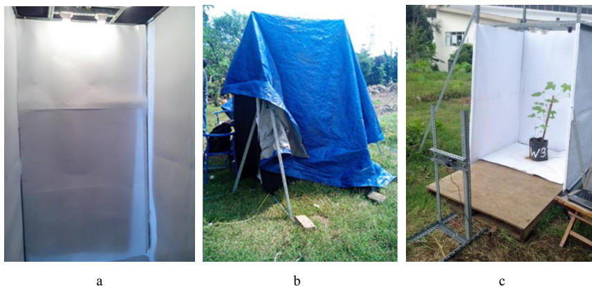
Fig 2. (a) Inside area of image acquisition box; (b) outside area of image acquisition box; (c) soybean plant inside image acquisition box.
