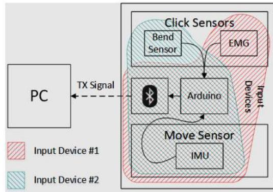
Fig. 2. Block diagram of input devices.
