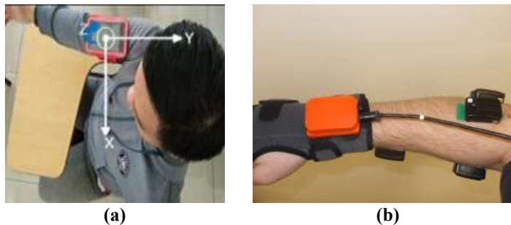
Fig. 1. a) Related work using sensor in smartphone and jerk of upper arm (top view); b) Related work using industrial IMU and EMG sensor attached on the forearm
