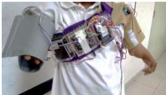
Fig. 12. Input device mounted on the torso and lower arm of a physically impaired subject
