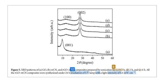
the mCN. However, the rGO-mCN obtained under 4 h of sonication time showed a slight decrease in diffraction intensity as compared to the mCN. This might indicate that the prolonged sonication time would affect the ordered graphitic structure of the mCN but it did not give a significant effect on the photocatalytic performance of the composite sample.
