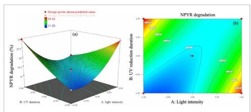
$\textbf{Figure 7.} \ Effect of interaction between the light intensity and the UV reduction time expressed in (a) 3D response surface and (b) contour plot with the GO loading was kept constant at 5 wt%.$
