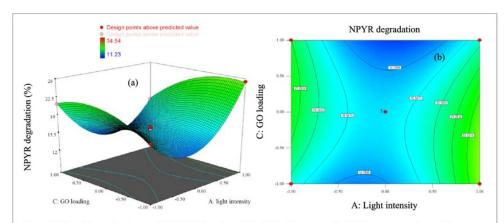
$\textbf{Figure 8.} \ Effect of interaction between the UV light intensity and the GO loading expressed in (a) 3D response surface and (b) contour plot with UV reduction duration kept constant at 12 h. \\$
