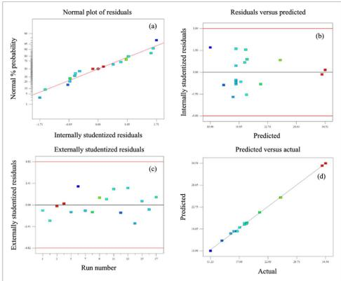
Figure 6. Diagnostic plots for evaluation of the adequacy, (a) normality, (b) internally studentized residuals, (c) externally studentized residuals, and (d) actual and predicted NPYR degradation.
