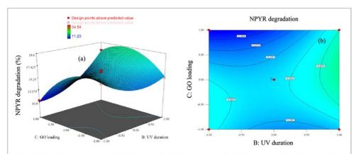
Figure 9. Effect of interaction between the UV duration and the GO loading expressed in (a) 3D response surface and (b) contour plot with UV light intensity kept constant at  $8 \text{ mW cm}^{-2}$ .
