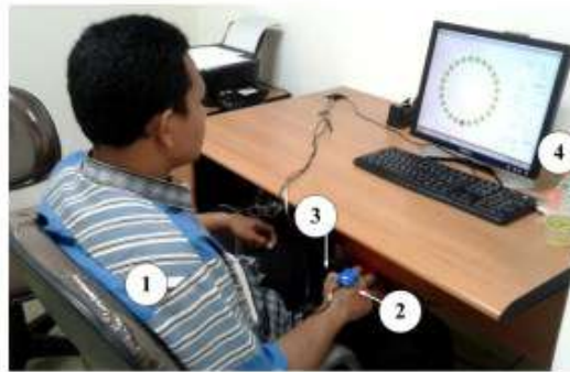
Figure 3: Illustration of experimental conditions: 1) Subject (0.9 m from display); 2) Inertial sensor (mounted on the back of the dominant hand); 3) Click part (grasped with the dominant hand); 4) Display (computer monitor)
