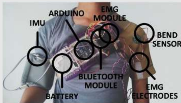
Fig. 8. Input devices mounted on the torso and lower arm, including labels for all device parts
