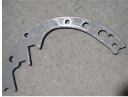
Gambar 3. Elemen brake shoe : stang
