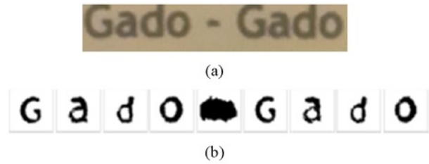
Fig. 6. (a) Cropped image that received by server; (b) Results of preprocessing
