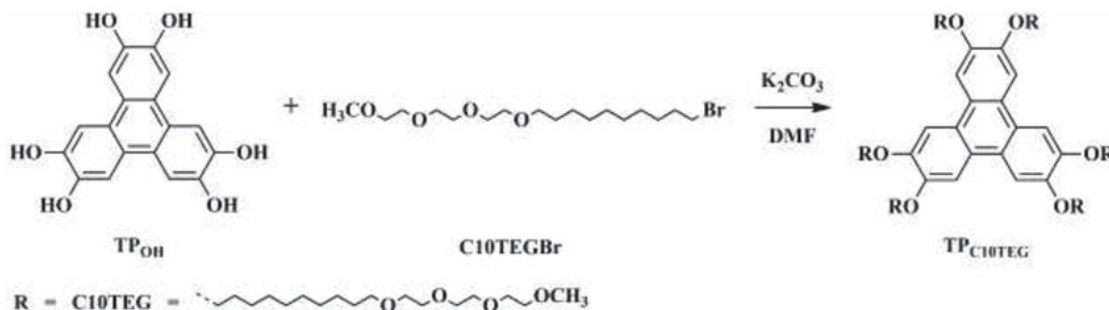
FIGURE 1. Synthesis and molecular structure of amphiphilic triphenylene bearing decoxy triethylene glycol ( \text{TP}_{\text{C10TEG}} ) from Williamson ether substitution reaction between 2,3,6,7,10,11-hexahydroxytriphenylene ( \text{TP}_{\text{OH}} ) and amphiphilic decoxy triethylene glycol bromide ( \text{C10TEGBr} ) as shown in reference [11].
